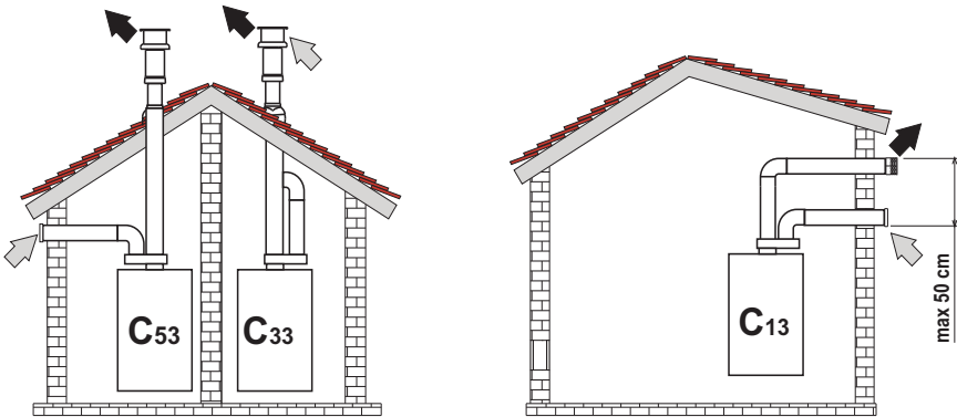
fig. 25- Examples of connection with separate pipes
